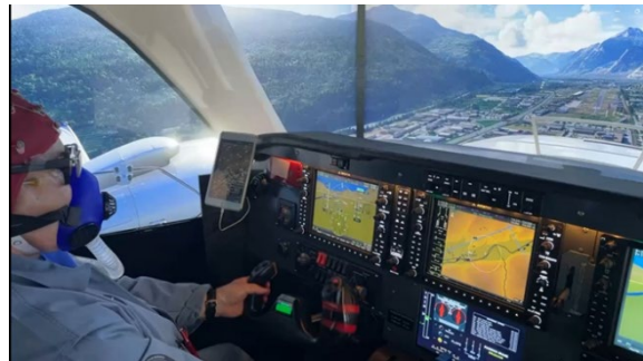
View of Main Panel Glass Cockpit GARMIN 1000
